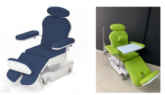
Arsimed Panamera Dialysis Chair is designed for dialysis, oncology, chemotherapy. The chair consists with 3 main parts. Back rest, seat part and leg rest. The chair makes back up&down, chair up&down, leg rest up&down, cramp support and trendelenburg&reverse trendelenburg movements by 5 DC motors with using hand control.
